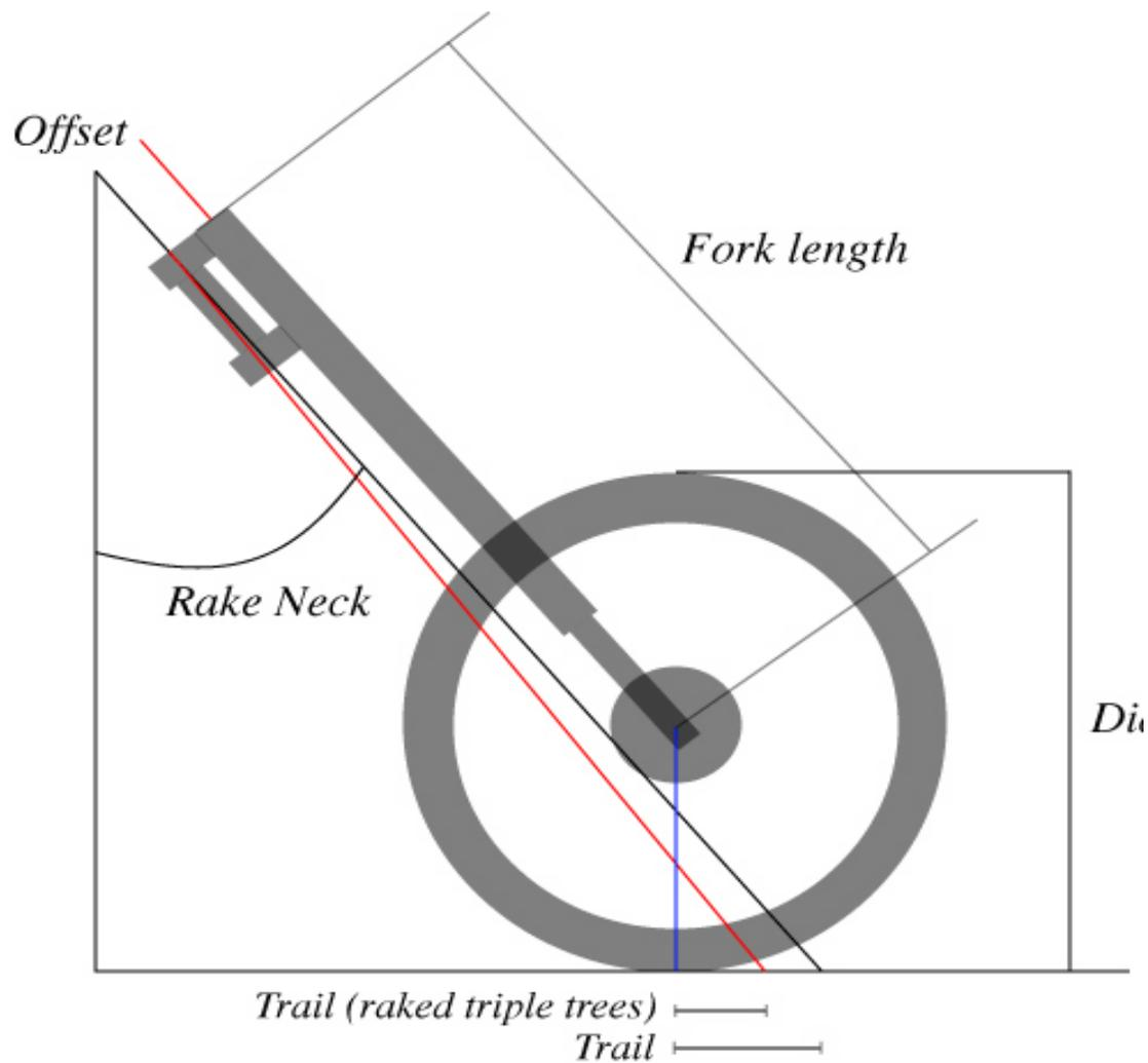
5. The trail is the distance in inches between the axle vertical centerline and the point where the straight edge touches the ground, (distance between A and B in diagram). Keep the straight edge and the carpenter's square in the same position and measure the distance in inches between these two points at ground level.
